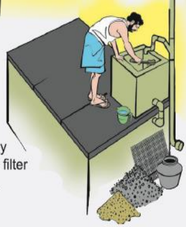
Cleaning the sump/tank once in six months or earlier depending upon the need.
